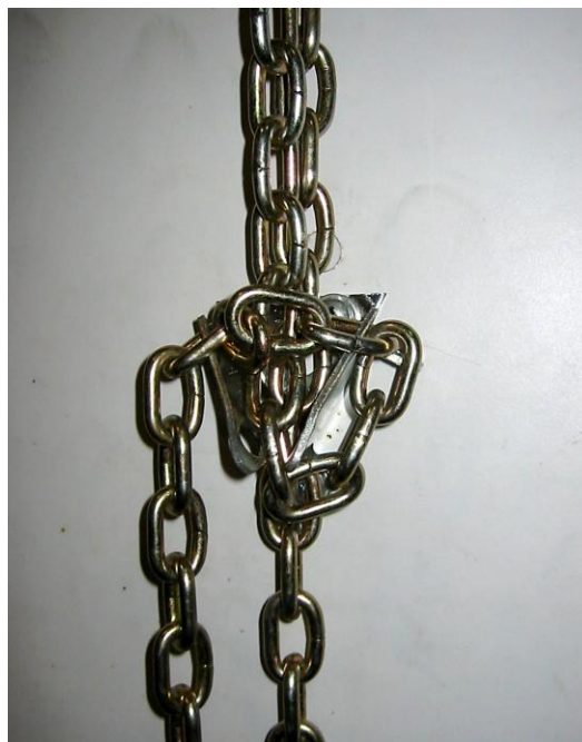
Photo #18 (Hoist Chain Locking)
