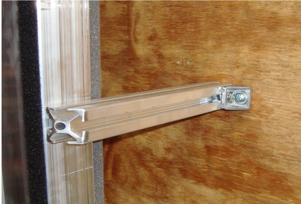
Photo #7 (Mid Support Bar Mounting)
