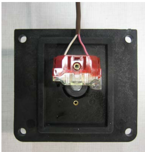
Photo #36 (Pullcord Switch Station Wiring)
