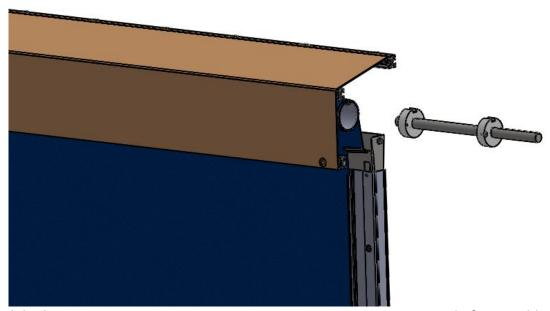
2. Slide the Header Mounting Bracket, with 1" bore Bearing, onto the Drive Shaft Assembly.
