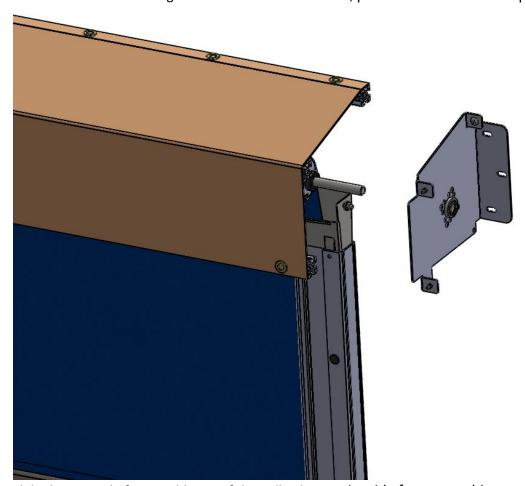
9. Slide the Drive Shaft Assembly out of the Roll Tube, put it aside for return shipment.
