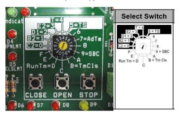
Press the "Open" button and allow the door to reach the fully opened position. The MRT is now set. Immediately proceed to the next step.
