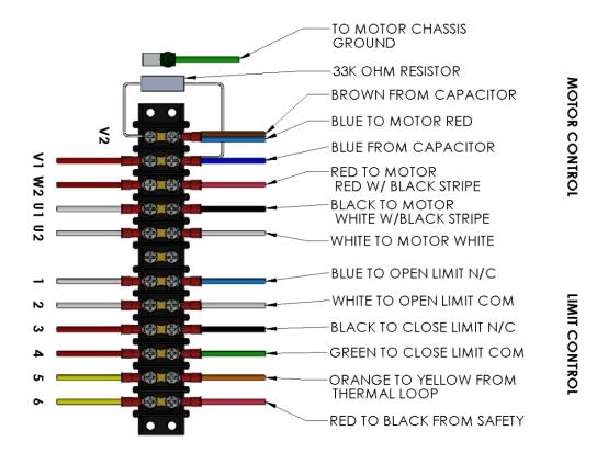
The following schematic shows your Motor and Limit Control wire connection points within the control panel:
