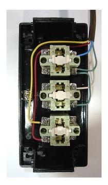
Route the cable through one of the station knockouts and carefully reinstall the cover. Make sure that the cover is installed properly and that the buttons work freely.
