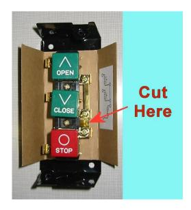
Connect the wires as shown in the following photo. Note that the yellow and red wires go to the N/C terminals on the Stop button
