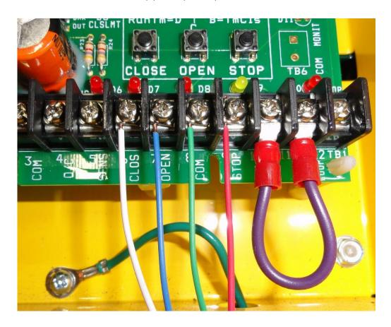
Single-station control installations are performed by simply running the control wiring between the control station and the operator, and attaching the appropriate wires to the screw terminals as indicated in the following photos:
