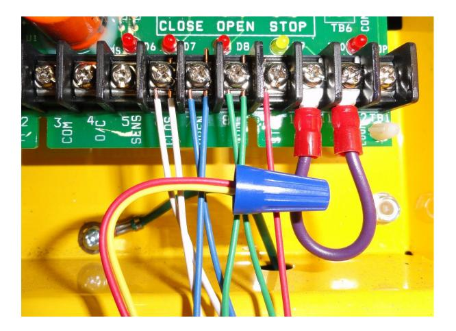
The wiring for the additional control station is now complete. You can continue to add control stations by following this same procedure. Connect the blue, white, and green wires to the corresponding terminals in the operator. Disconnect the red wire from the previous station from the #9 Terminal, connect it to the yellow wire for the new station (wire nut), and connect the red wire for the new station to Terminal #9.
