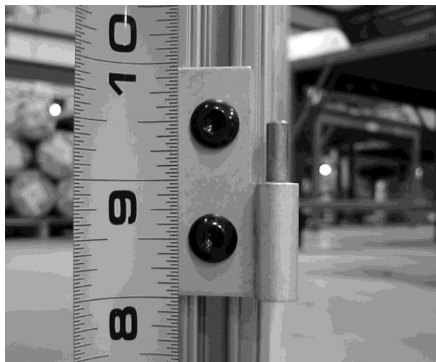
Photo #4 (Short Hinge Pin Installation)
