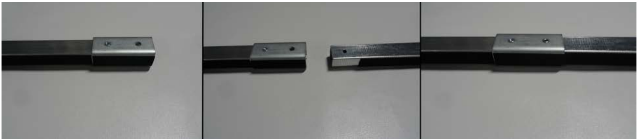
Photo #3 (Track Splice)
