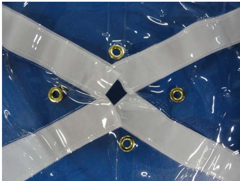
Photo #14 (Joined Panels at Topper peak)
